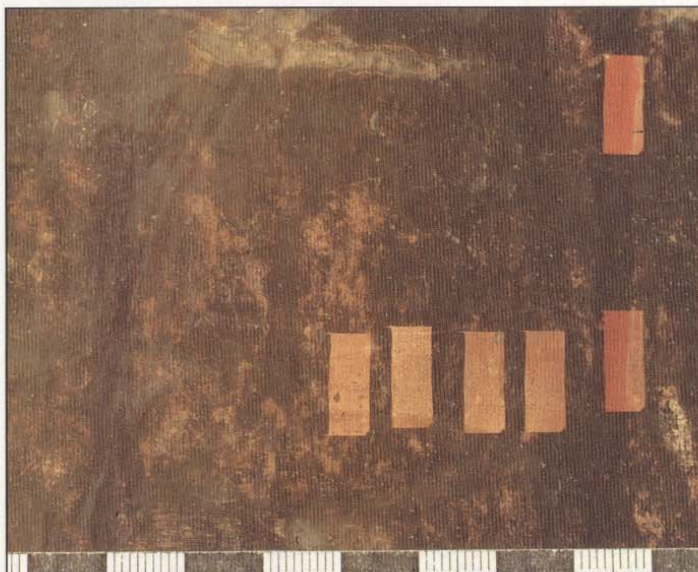
The art of using the laser system is to adjust the power density, repetition rate and velocity of the beam across the surface so that dirt is removed without damaging the underlying paint and the subsurface. ©Thomas Haupt.
